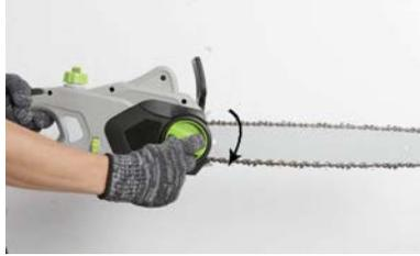
The chain is correctly tensioned when there is no sag on the underside of the guide bar, the chain is snug, but it can be turned by hand without binding.
