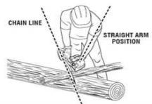
Keep the unit running the entire time you are cutting, maintain a steady speed.
