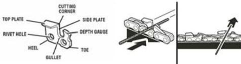
Lift file away from the steel on each return stroke.
