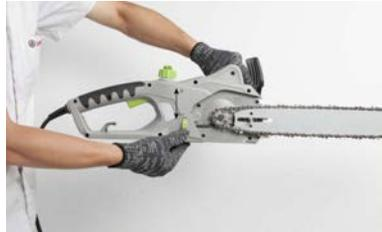
**NOTE:** A new chain tends to stretch, check chain tension frequently and tension as required.
