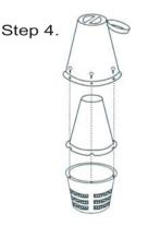
Place the green outer cone over the black inner cone, making sure that the lid opens in a convenient direction. Line up the screw holes in the base of the green outer cone with the notches on the base of the black inner cone. Use six 10x5/8 self tapping screws to secure the cones to the basket.
