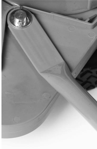
Fit the lower section of the handle over the handle posts on either side of the mower. Then place the washer over the post, insert the cotter pin and bend its ends back over the post as shown in above left photo. Continue assembly of the middle and top sections of the handle using the handle bolts and wing nuts as shown in above right photo.
