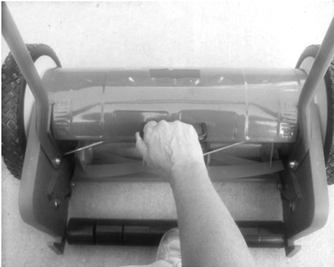
The cutting height of the IDEAL may be adjusted from approximately 1.5 inch up to approximately 3.5 inches. Actual height may vary according to the density of the turf. Adjust the mower to the desired height first by rocking the handle forward so that it is sitting on the ground and the mower is upside down. The black height adjustment knobs are on the right and left of the mower body.
