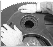
7. Place a 1/2" washer onto the shaft so it is up against the outside of the cradle, and then secure by placing the cotter pin through the hole at the end of the shaft. Use pliers to bend the legs of the cotter pin so the pin is secured.
